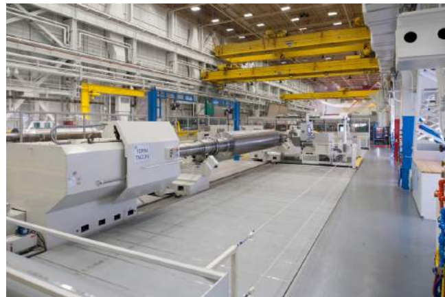
Horizontal lathes for generator shafts
