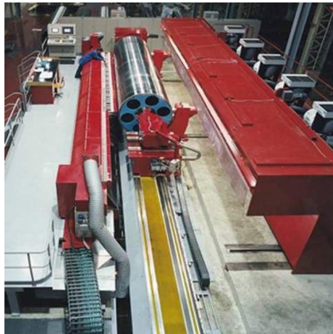
Multiple drilling machines for suction rolls
