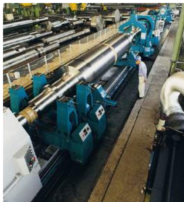
Deep hole drilling machines for generator shafts
