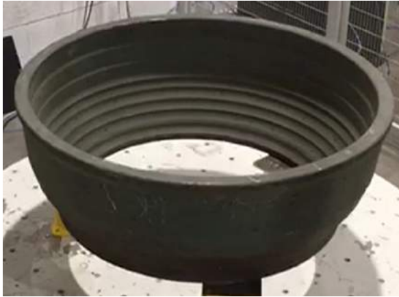
Raw forged part (uneven condition and stock)
