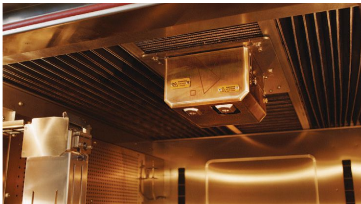
Double extruders mean double the print speed. (Provided by Roboze)
