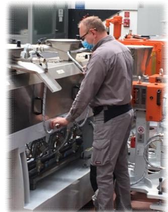
The screw profile is optimized to process various families of polyolefin waste, following intensive **software simulation, modelling** and **granulation tests** in the new technology laboratory constructed recently with state-of-the-art compounding lines.
